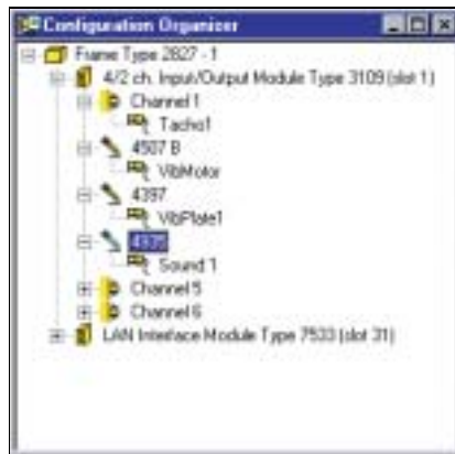
Fig. 2 Configuration Organiser showing the front-end, modules, transducers and signals in a configuration for a measurement task using a single front-end
